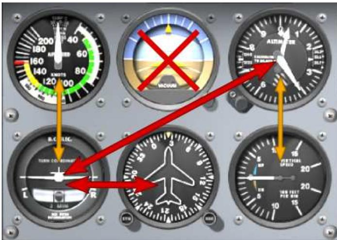
Example of instrument scan, leaving out the attitude indicator
